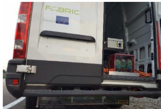
Figure 42. General specifications of the DWPT charger (left) and view of the van prototype on the experimental road (receiver and on board DC/DC converter can be seen) (right).
