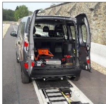
Figure 34. General specifications of the DWPT charger (left) and view of one car prototype on the experimental road (one cover has been removed and road embedded components can be seen) (right).
