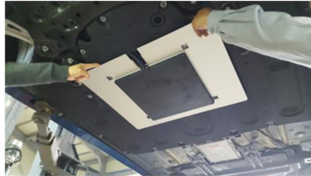
Figure 17. KEPCO and Green Power Co. general specification of WPT charger prototype and (right) WPT charge vehicle adaptor attached at the bottom of commercial EV (IONIQ).
