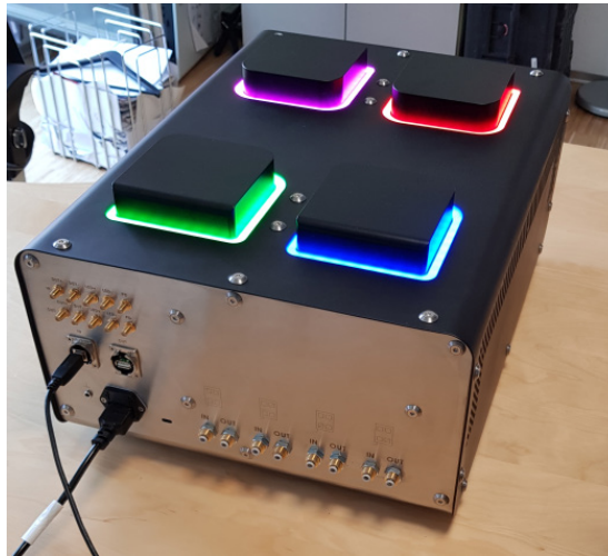
Figure 5: Litos instrument with color indicators around each measurement chamber showing the operating condition (green: setpoint reached, blue: measurement running, red: error or warning, magenta: trying to reach a setpoint).
