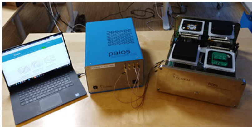
Figure 2: Picture of the tabletop setup including the laptop, the all-in-one characterization instrument Paios and the stress test platform Litos, the latter being developed in this P+D project. The black Litos chassis as well as 2 chamber covers are removed here.
