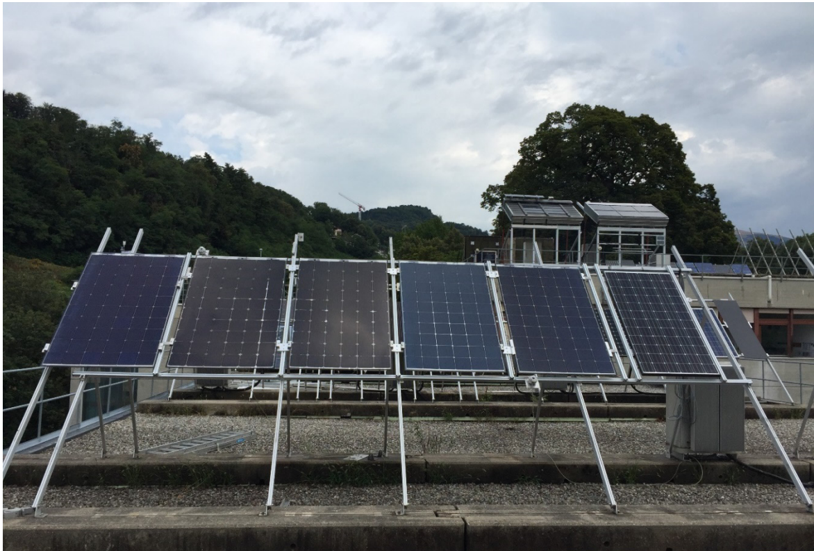
Figure 30: Picture of the test stand for bi-facial modules
