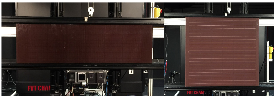
Figure 3: Two different PV modules with terracotta appearance: (left) C13-F1 module with prismatic glass and (right) C13-I1 module.
