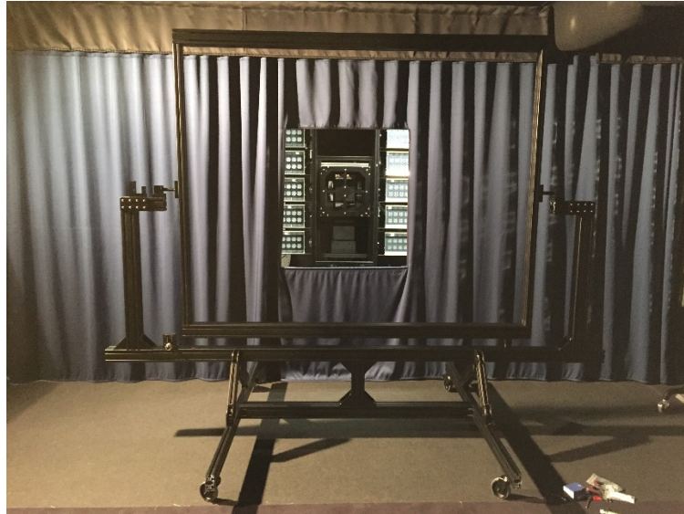
Figure 48: Rack mounting structure for the angular loss analysis of PV modules in sizes up to 1.5 x 2.0 m2
