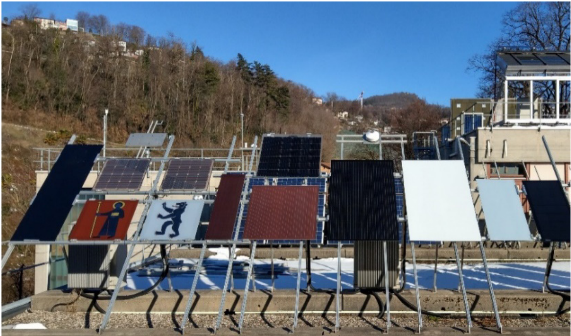
Figure 29: Picture of the test stand for aesthetic modules
