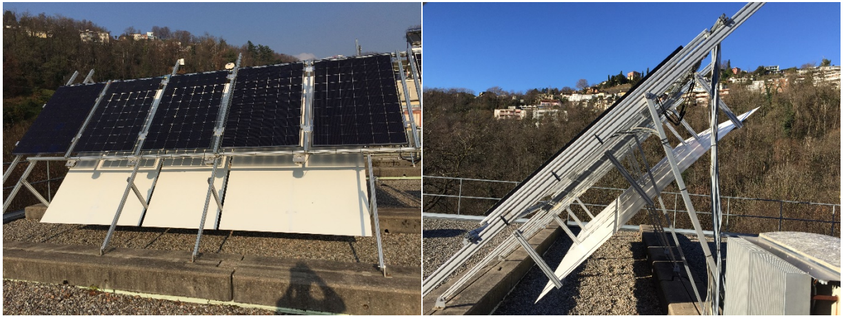
Figure 44: White diffuse reflectors mounted in the rear of bi-facial PV modules: front (left) and side (right) view.
