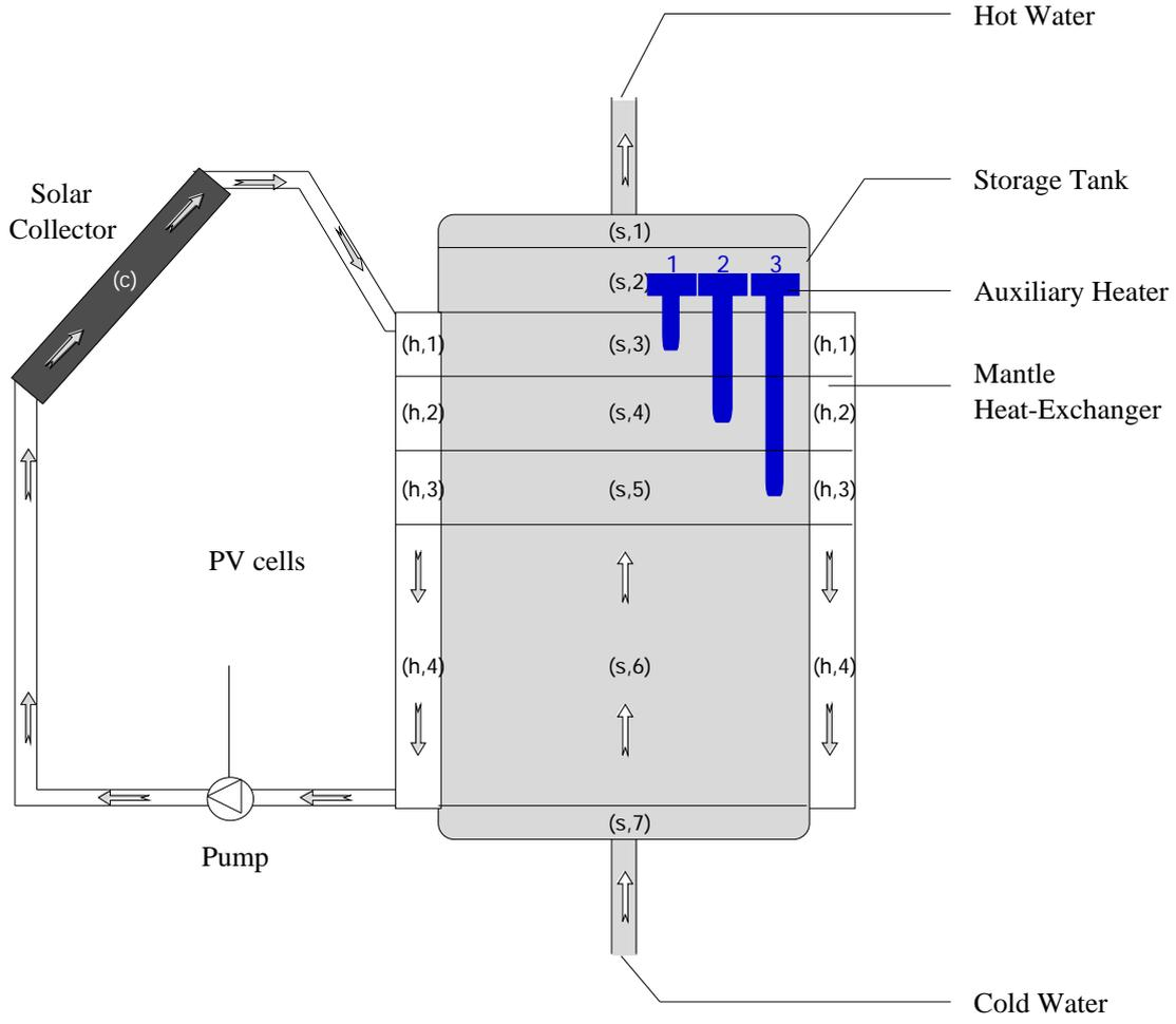
Figure 1: Model of the SDHWS
