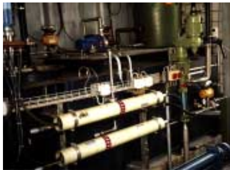
RO plant in Otelfingen, Switzerland, treating the effluent of solid waste digestion
