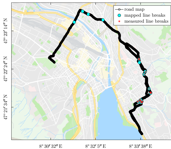
Figure 11: The road map as present on 24.05.2019 at 11:58. The colored nodes indicate the line breaks that were mapped in previous runs. The red asterisks show the measured line breaks on 24.05.2019 between 11:50 and 12:50. Note that the vehicle was not driving on the entire road map during this time period.
