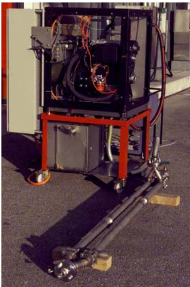
Figure 2. The cogeneration unit
