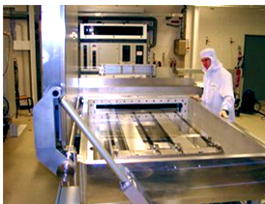
Figure 1: Industrial KAI plasma deposition plant (Photo: Unaxis)
