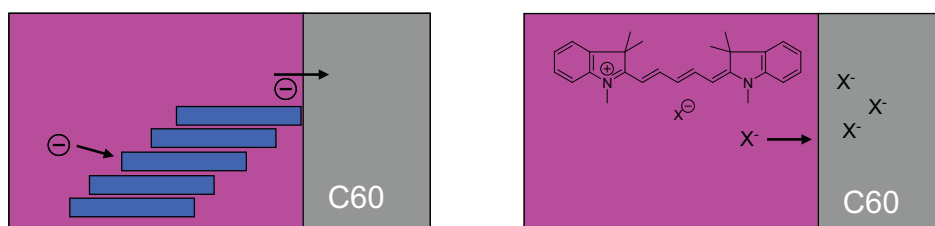
Fig. 4. Left: Schematic of a cyanine aggregate (blue bars) on a C_{60} layer. Right: Chemical structure of a cyanine dye with counter anions ( X^- ) and C_{60} layer. The positive charge of the cyanine chromophore is balanced by counter anions. These anions are mobile and are displaced into adjacent layers.
