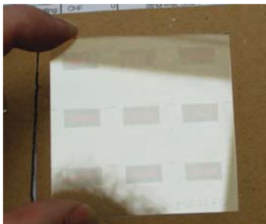
Picture of a 10x10 cm FTO22-15 glass having 9 screen printed reference electrodes.
