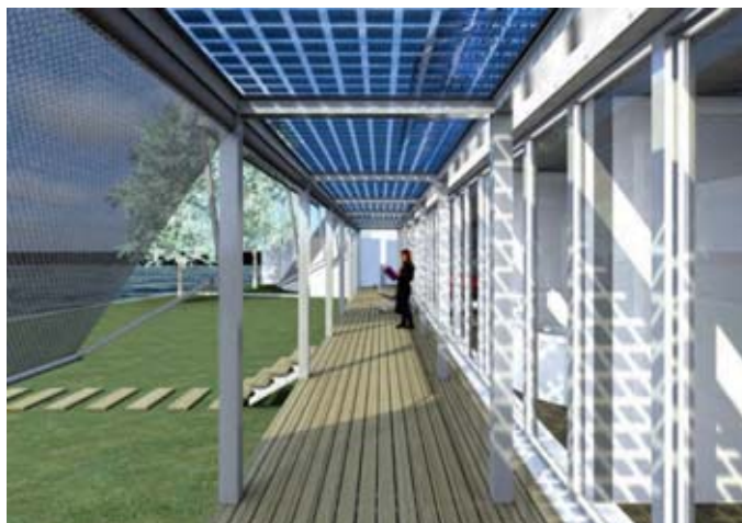
Figure : ArchiCAD rendering of a BiPV sun shading element, the design as refined with the software Houdini Source: Isa Zanetti, ISAAC-DACD-SUPSI
