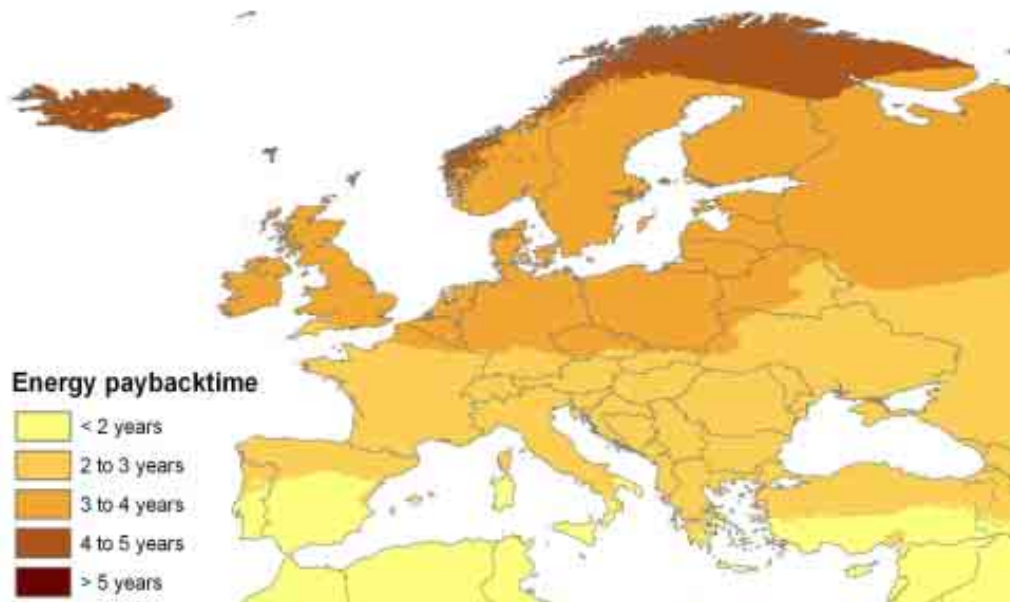
Fig. 5: Energy pay back time of 3\text{ kW}_p slanted-roof multicrystalline panels operated in Europe in relation to the UCTE electricity mix (own calculation with [11])
