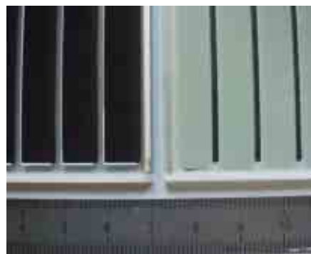
Close-up view of the monolithic dye solar cell module before dye impregnation
