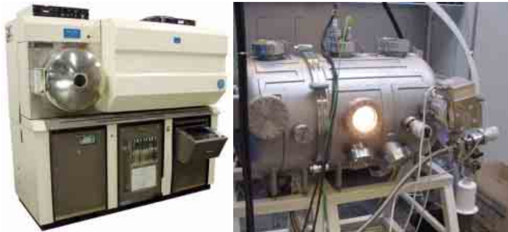
Figure 1: Vacuum deposition equipments used for upscaling of process steps: Inline Sputtering equipment (Material Research Corporation) and absorber layer evaporator system (custom build vacuum chamber and evaporation components)
