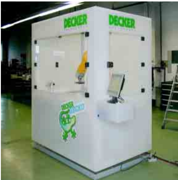
Figure 2: Prototype built for demonstrating singulation capability of thin wafers
