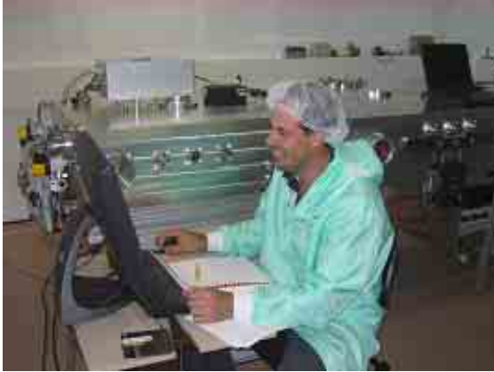
Fig. 5: picture of large area KAI-M cluster deposition tool with one operational chamber.
