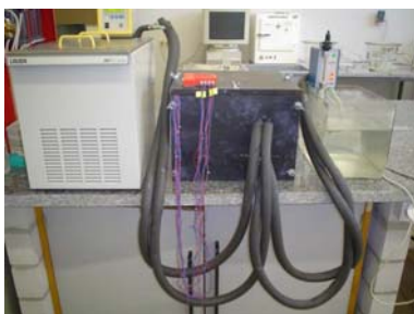
Figure 5: thermal baths to measure thermal conductivity
