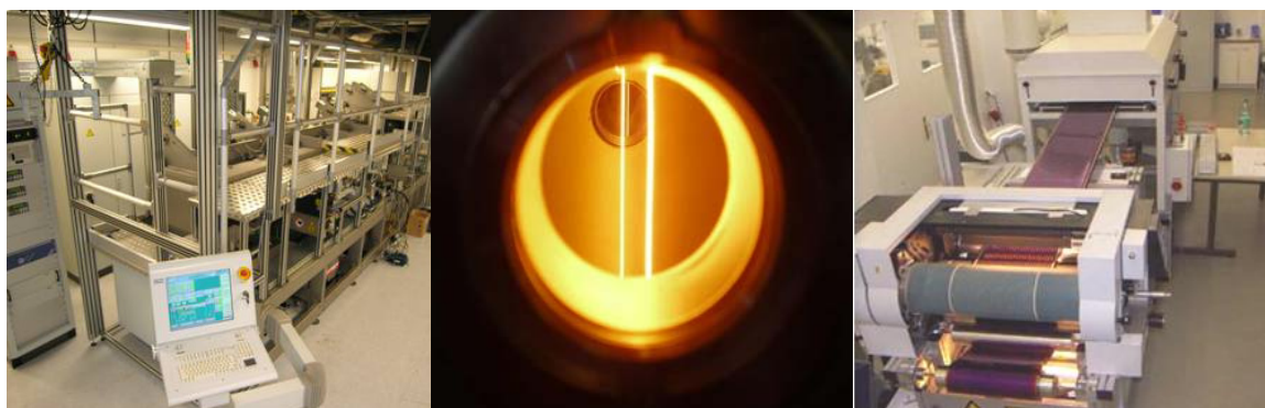
Figure 1: (left) New MW-PECVD roll-to-roll system built by the system manufacturer R&R and now used at ECN, (Middle) New large area HWCVD system at the UBA, (right) Roll-to-roll production line at VHF-Technologies.
