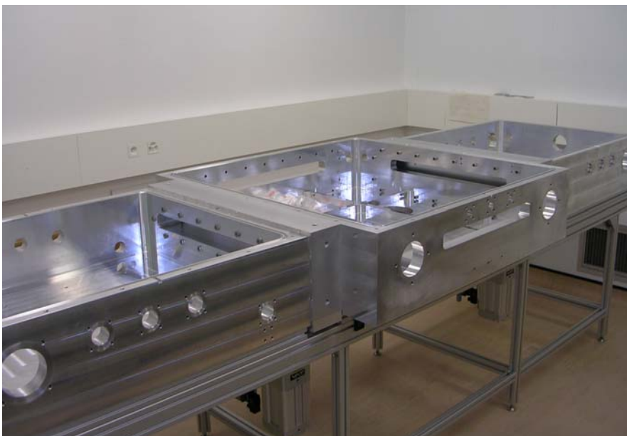
Fig. 7: Picture of the assembly of the new double chamber deposition system with KAI-M plasma box from OC Oerlikon. The load-lock chamber is in-between the two deposition chambers.
