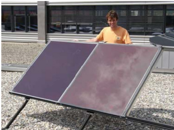
Fig. 3: AFG a-Si:H p-i-n module (1.4 m 2 ) on the right hand side and LP-CVD ZnO front a-Si:H p-i-n module on the left hand side. Note the darker appearance of the ZnO, which reflects the improved light trapping compared to AFG.
