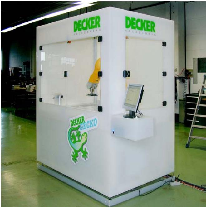
Figure 4: GECKO: a thin wafer singulation unit
