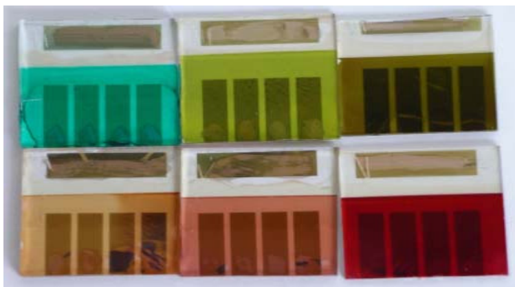
Fig. 2: Various solid-state dye-sensitized solar cells with solar efficiencies up to 4%. Top left: blue dye, \eta = 1.5\% ; top centre and right: zinc porphyrin dyes, \eta = 2.5 - 3\% ; bottom left: perylene dye, low \eta = \text{low} ; centre: Z-907 dye, \eta = 4\% ; right: indoline dye, \eta \rightarrow 4\% .
