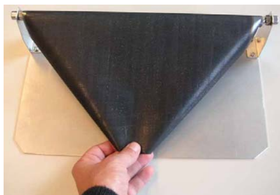
Figure 3: Pictures of flexible CIGS solar cell layers on a roll (left) and flexible mini-module to run a ventilator-fan.
