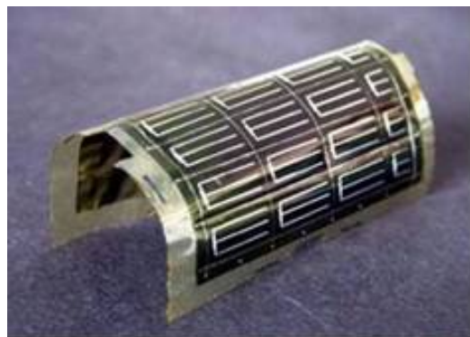
Figure 1: Flexible CIGS solar cells on a 5 x 5 cm 2 polyimide foil (left) and current-voltage characteristic of the 14.1% efficiency cell measured under simulated AM1.5 standard test conditions at ISE-Fhg Freiburg, Germany (right). This value achieved in December 2004 still remains the highest efficiency record for any kind of solar cell grown on polymer foil.
