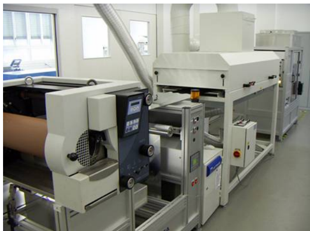
Fig. 3: New roll-to-roll production line at VHF-Technologies
