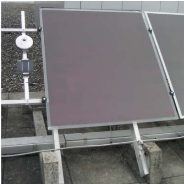
Fig 2 AFG a-Si:H p-i-n module of 1.4 m 2 area on the outdoor test bench of NTB (Neues Technikum Buchs).
