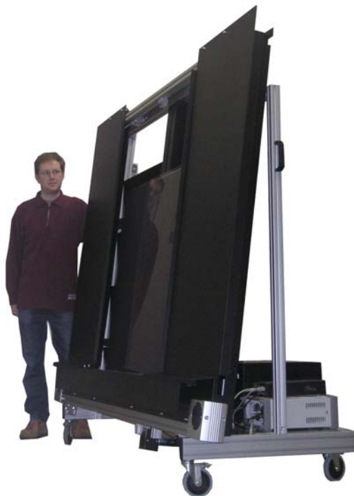
Fig. 5 Spectral Response Measurement System loaded with a 1.4m 2 monolithic series connected a-Si:H p-i-n module
