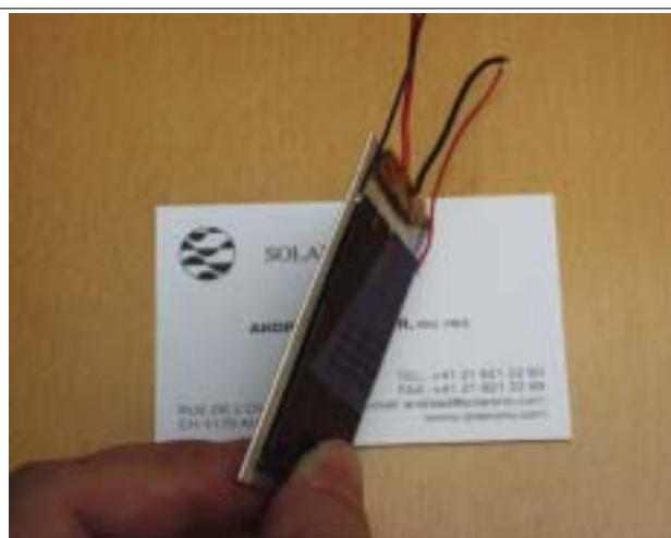
Assembled prototype Proto v1 (wires are provided to measure charging conditions)
