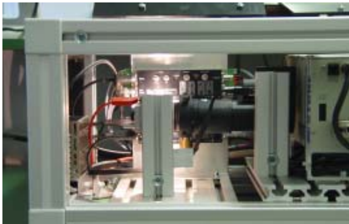
Figure 4b: Photograph of the light source feeding the input of the monochromator (right corner). In the background the lock-in amplifiers are seen.
