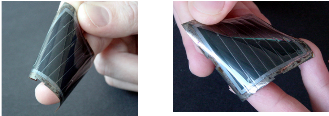
Figure 7: Monolithically interconnected flexible CIGS mini-modules on polyimide developed in collaboration with ZSW.
