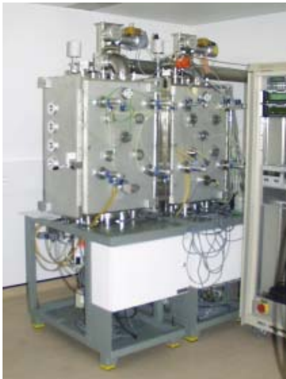
Figure 1: Large area single-chamber VHF- (81.36 MHz) deposition system at IMT. One chamber (left) serves as a load-lock as well as a doping chamber while the second chamber (right) is used for intrinsic layer deposition. Both chambers may accept substrates with size up to 30 \times 30 \text{ cm}^2 .
