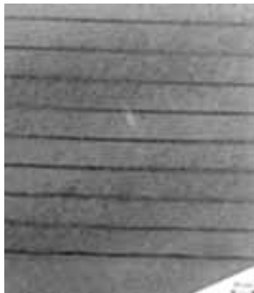
Fig. 7: TEM images of two UHV-CVD grown SiGe structures: Detailed view of a structure with 30 SiGe quantum wells with 3 nm thickness and 25 % Ge content (left) and a wavelike layer structure of 10 SiGe layers with 5 nm thickness and 35 % Ge content (right).
