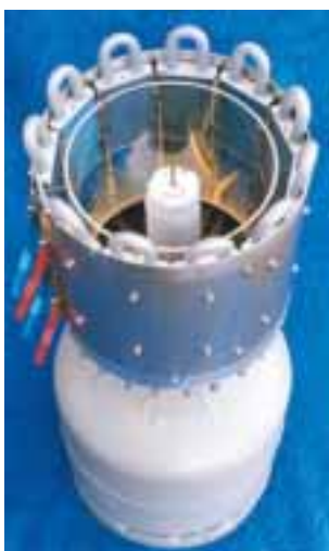
Fig. 1: TPV prototype system with \text{Yb}_2\text{O}_3 emitter and silicon photocells. The upper reflector is removed.
