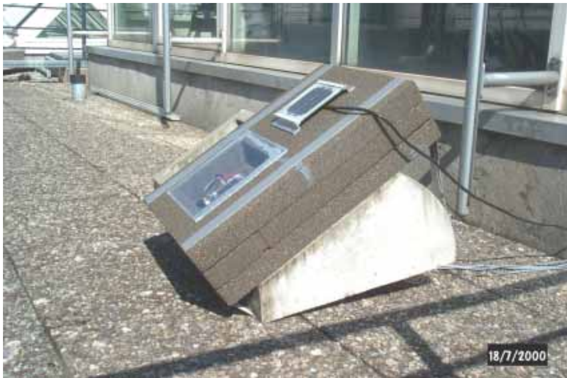
Figure 3. : prototype of the a-Si collector with foam glass insulation and single extra-white glazing.
