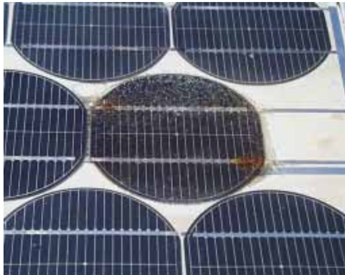
Picture 4: delamination on one cell (major defect) in a module of string 6.
