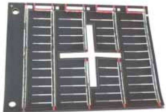
Fig. 2. One submodule consists of 4 serially connected solar cells. The cross in the middle is left open in order to allow the antenna to radiate.
