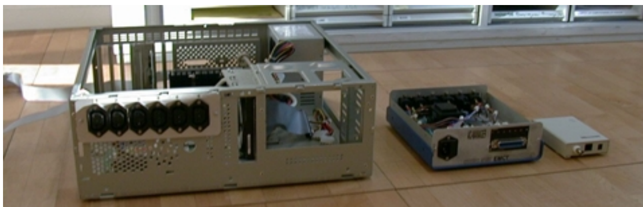
Fig. 4.3: Linux computer with integrated control unit; separate controller with 8 switching outputs; LAN interface card (from left to right; view from front)
