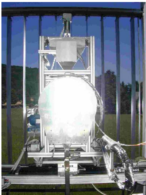
Fig. 3: The indirect-heated solar lime reactor operated with concentrated solar energy. Front view of reactor with open shutter (left); rear view of reactor with parabolic dish (right).
