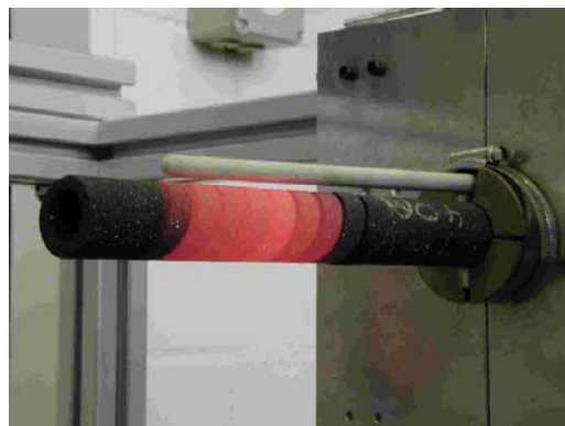
Fig. 4b: SiC heating element working "in air" during a test. On top of the red glowing coil, the white platinum thermocouple is placed.
