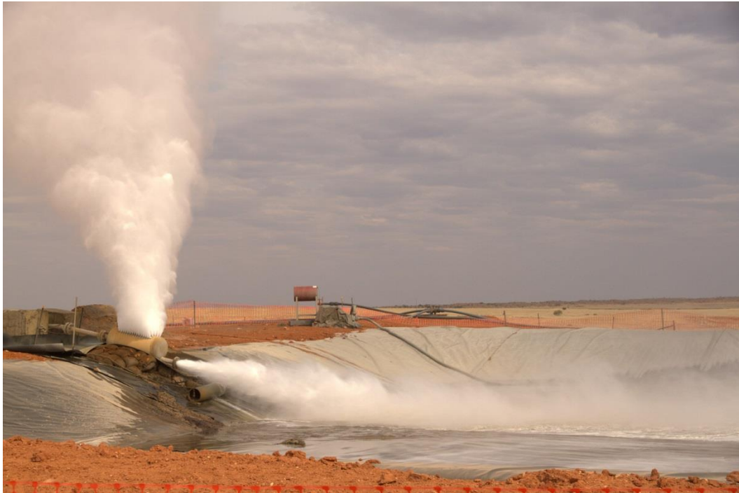
Figure 24.1 Clean-up flow from Habanero 4; flowrate 36 kg/s at a wellhead temperature about 200 °C and climbing. (Photo courtesy of Geodynamics Limited)
