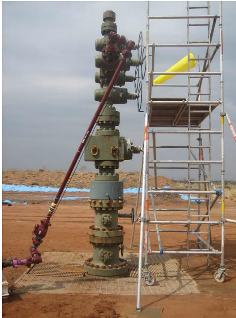
Figure 8.1 Petratherm's Paralana 2 wellhead, located in the northern Flinders Ranges of South Australia. Paralana 2 was the first deep well to test the geothermal resource at the Paralana field. (Photo courtesy of Petratherm)
