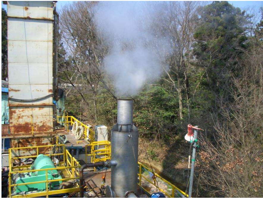
Figure 12.8 Well production test SD-1 in Sado, Niigata Prefecture, Japan. (Photo courtesy of A. Takaki)
