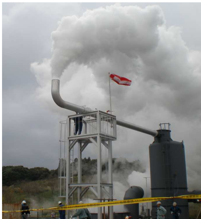
Figure 12.7 Production test of the N2I-IK-4 well, Ikedako-tobu, Kagoshima Prefecture, Japan. (Photo courtesy of A. Takaki)
