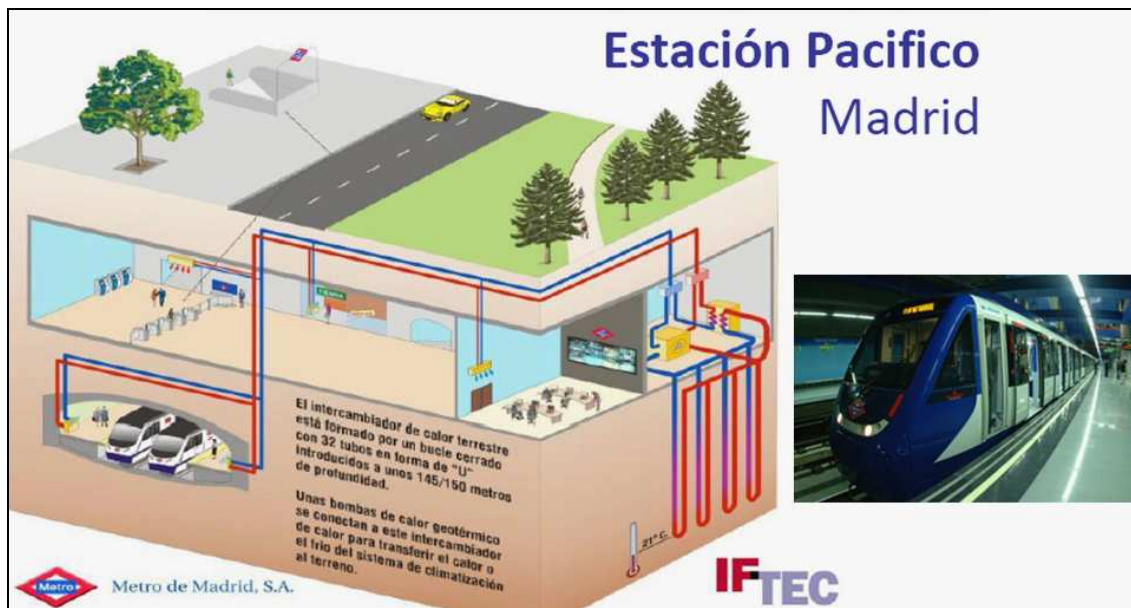
Figure 16.5 Geothermal heat pump installation in the Madrid Subway.
