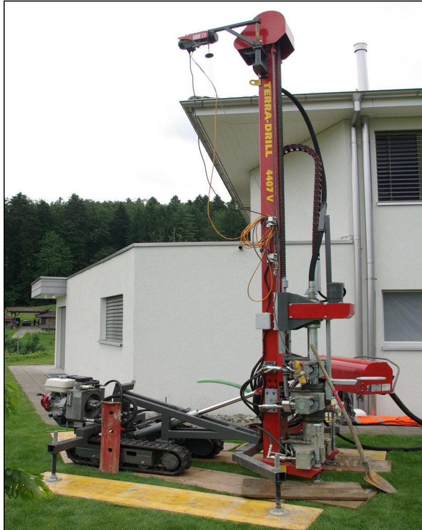
Light and compact mini-drill rig for drilling shallow (100-200 m) wells for GHPs in Switzerland. (Photo courtesy of Swiss Federal Office of Energy)
