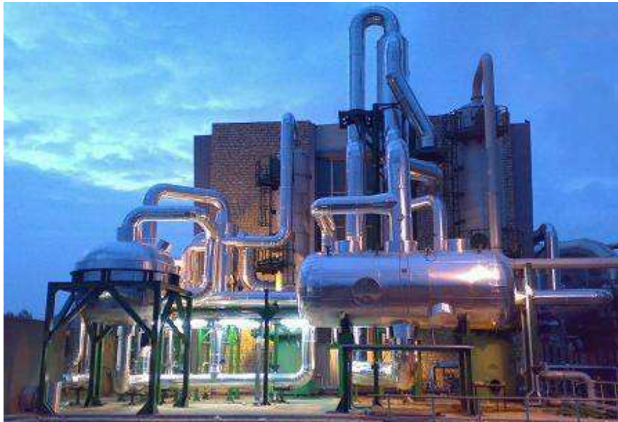
Figure 11.7 The AMIS plant for the Hg and H 2 S abatement installed at the 20 MW Nuova Gabbro power plant.
