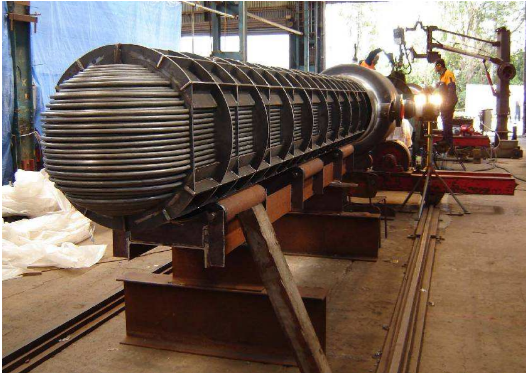
Figure 20.1 One of four high pressure heat exchangers being manufactured for the 1 MWe Habanero power station. (Photo courtesy Geodynamics)
