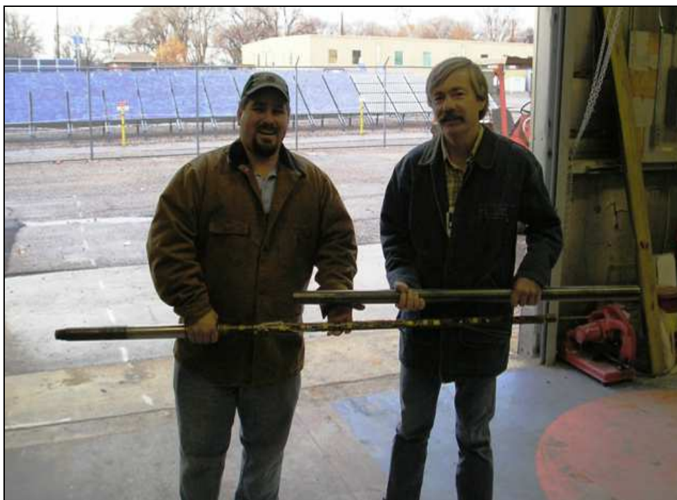
Sandia-developed precision pressure/temperature well monitoring tool that was fielded downhole at the Coso geothermal site for about 1 year. (Courtesy Sandia National Laboratories)
