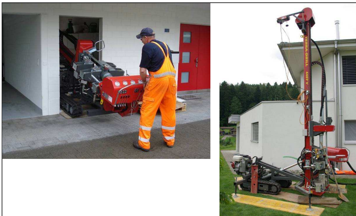
Figure 17.3 Light and compact mini-rig to drill shallow (100-120 m deep) wells for deployment of geothermal heat pumps systems. (Source: Terra AG and J. Wettstein)
