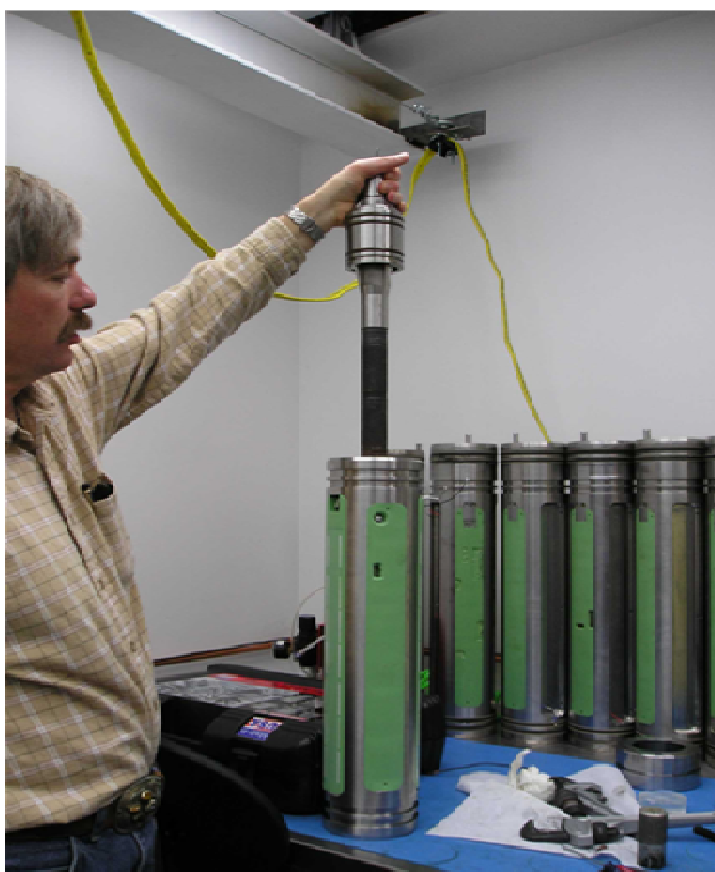
Sandia-developed telemetry package being assembled into one of Novetek's wired pipe subs. (Courtesy Sandia National Laboratories)
