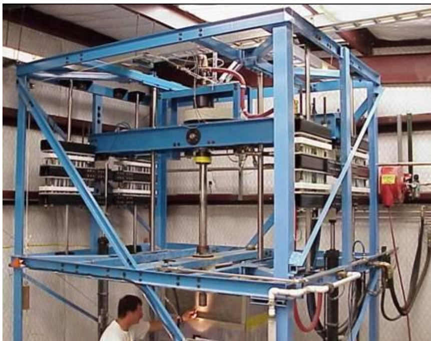
Figure 4.2 First generation realization of Drilling Dynamics Simulator in Sandia's Hard-Rock Drilling Facility (Raymond, et al. , 2007).
