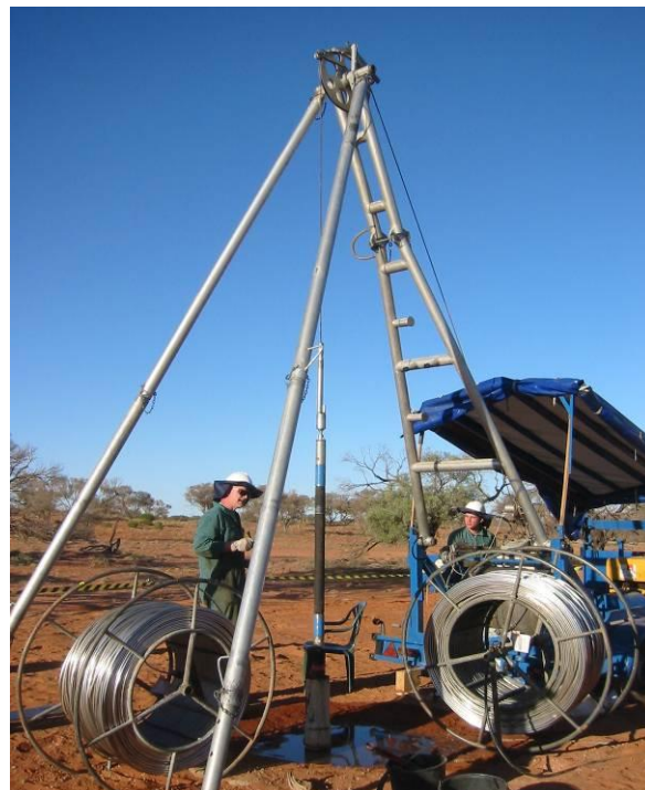
Figure 20.3 Hydraulic Fracture testing in Blanche No 1. exploratory well (by MeSy, Germany).
