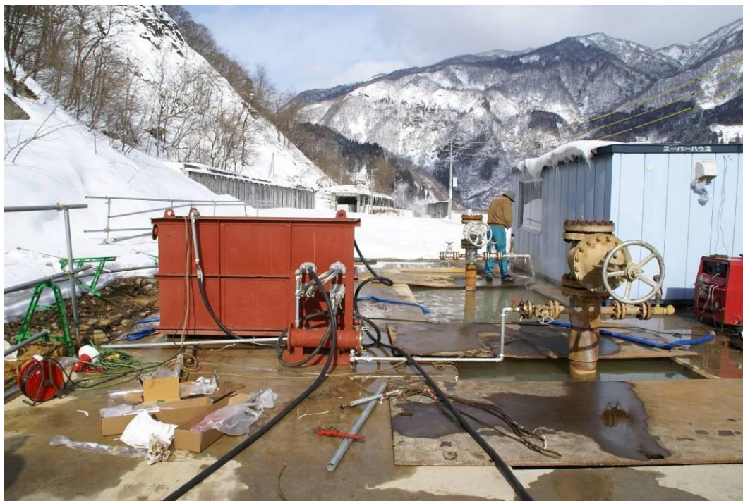
Figure 13.13 Carbonate scale evaluation lines including heat exchangers for the Hot Spring Ecogene System Project in Otari, Nagano Prefecture, Japan, on 20 January 2008 (courtesy of H. Muraoka).
