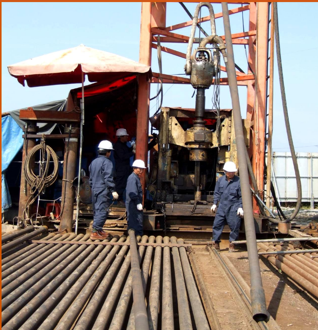
Tripping in at the 2 km deep well, Pohang, Republic of Korea (courtesy of M. Mongillo).
