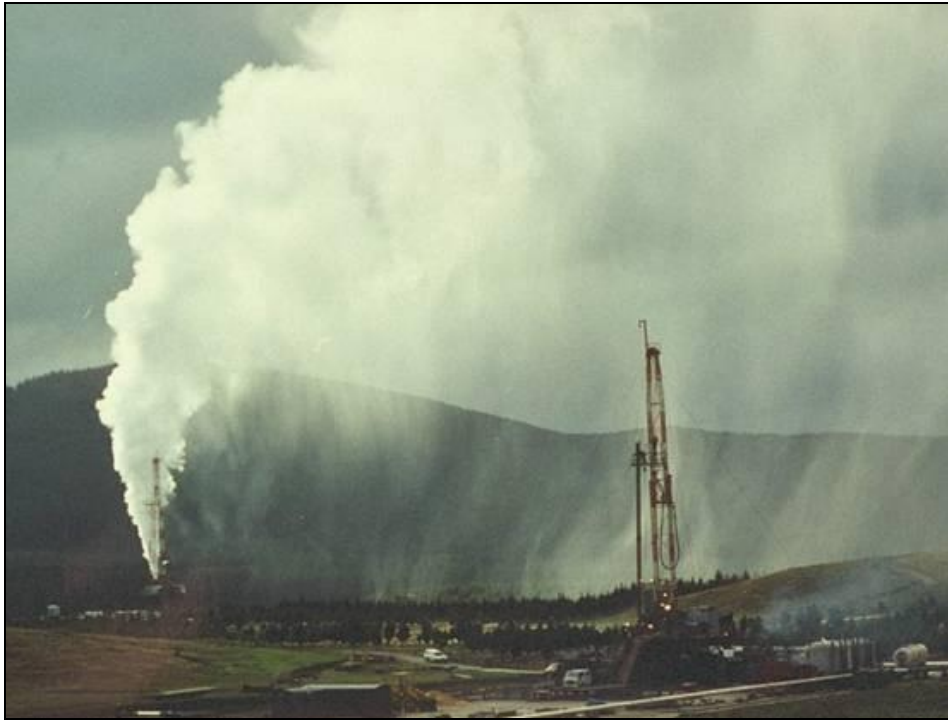
Figure 16.4 New well discharging vertically at Rotokawa Geothermal Field.
