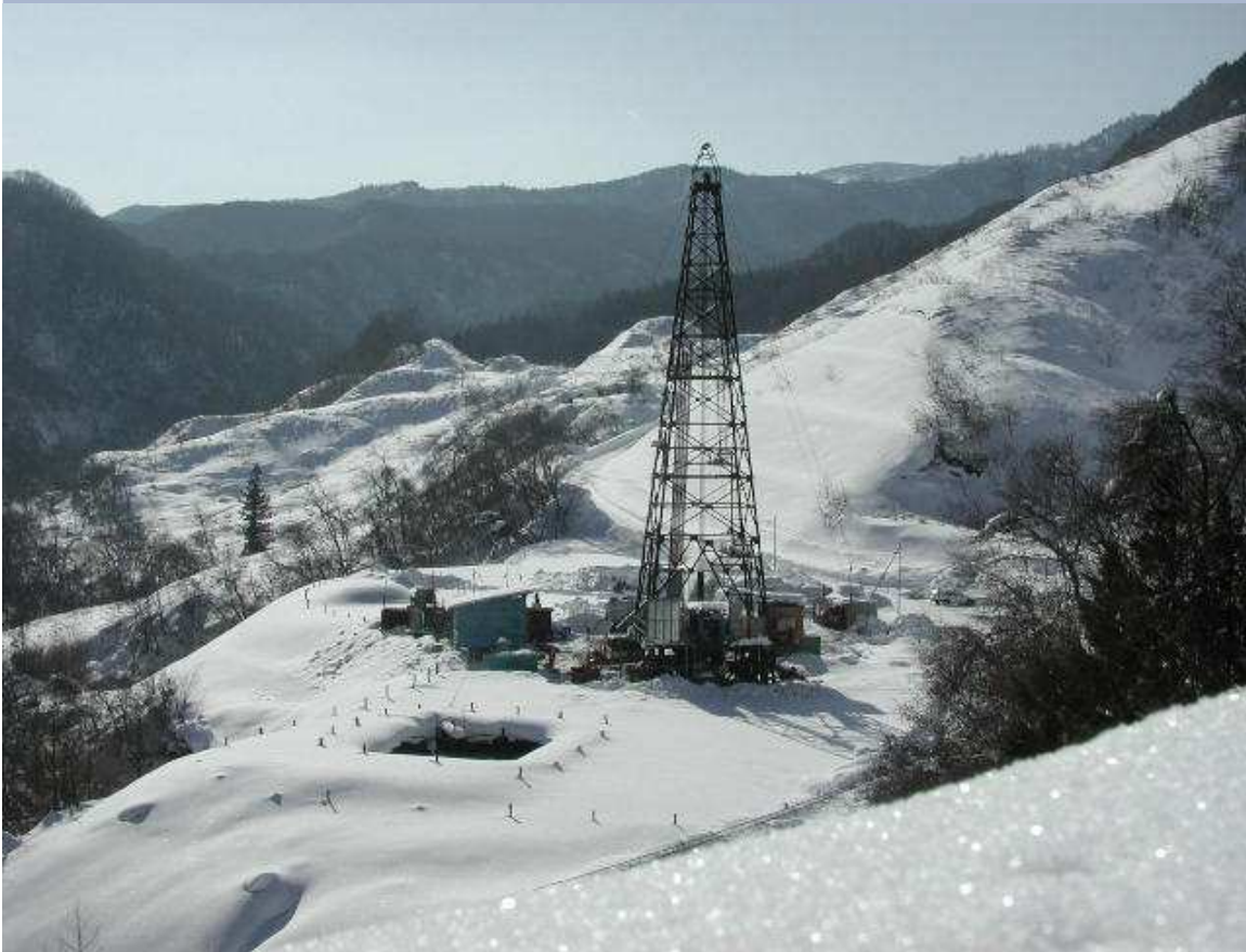
Well N16-TE-2 in Tenei Village, Fukushima Prefecture. The well was drilled to a depth of 1400.8 m and reached a temperature of 112.1 °C for a small-scale power development by NEDO from late 2004 to early 2005 (Photo by Yuko Kizaki, Geothermal Engineering Co., Ltd).
