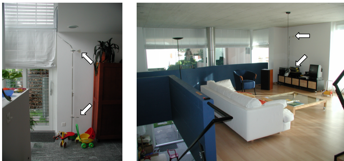
Fig. 2 Measurements of the air and surface temperature at the south-west wall in the living/dining room (left hand picture) and the living room at the first floor (right hand picture)
