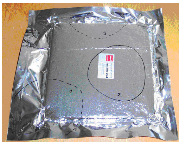
Figure 44: Sample preparation for the permeability measurements.
