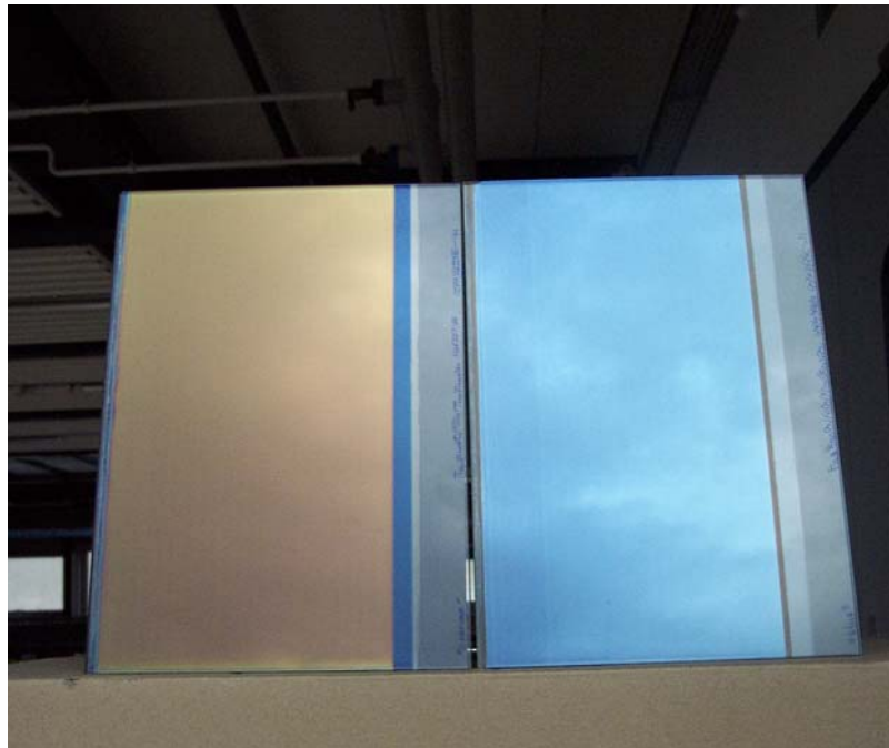
Fig.10: Sol-gel deposition of nanocomposite oxide coatings on A4 - sized substrates. (a) Photograph of glass panes coated with colored multilayer stacks. The loss in solar transmittance due to the colored coating amounts to only 1.4 percentage points (blue sample) and 3.4 percentage points (brownish sample). The optical data yield a visible reflectance of 14.0 % and 12.6 % for the blue and brownish sample, respectively.
