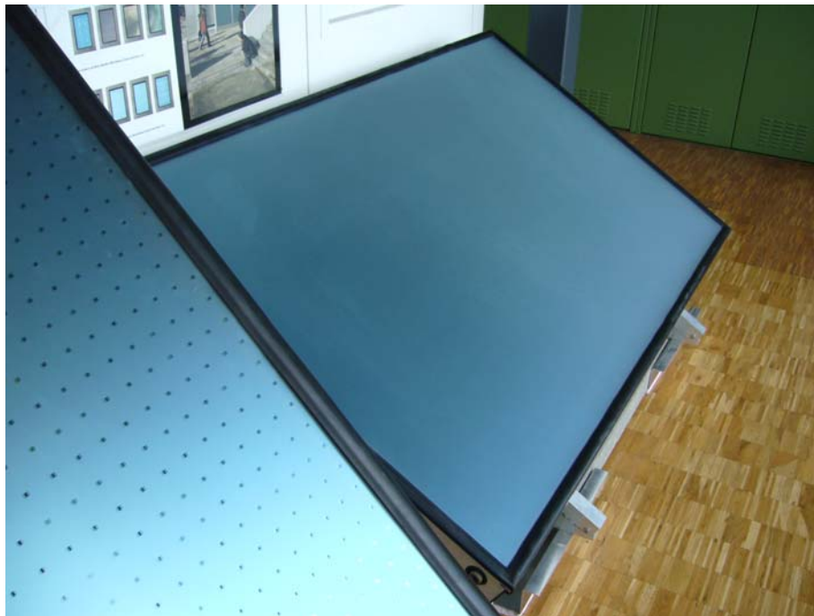
Fig.23: Solar collectors from SCHWEIZER covered with light blue glazing. An etching treatment has been applied on the outer side of the glass. The etched surface can be patterned on demand, giving a large freedom in design possibilities.
