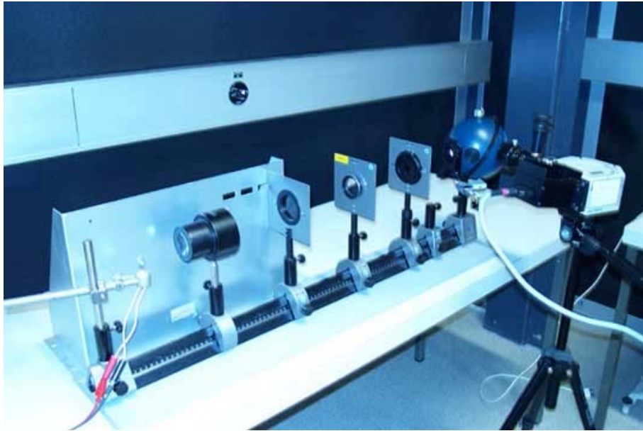
Figure 2.12: Integrating sphere, spectrophotometer and optical bench. The light emitted by a halogen lamp is collimated before reaching the integrating sphere.
