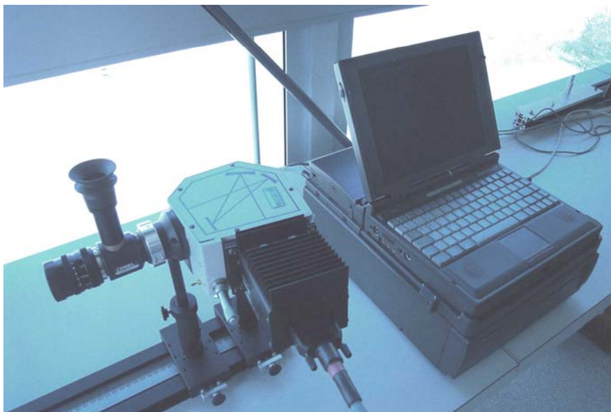
Figure 2.1: The spectrophotometer consisting of the sighting optics, the unit containing the dispersion optics and the detector. The photograph shows also the computer for the data acquisition (software “Instaspec II”).
