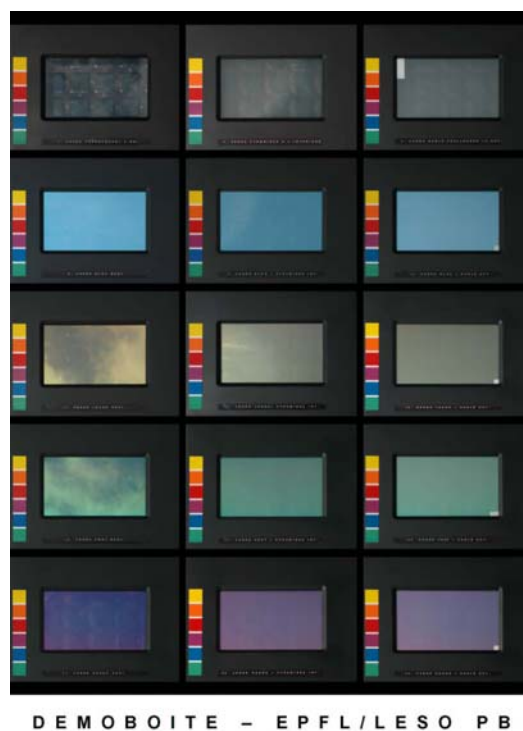
Fig. 8: Demonstration of various color shades and surface textures in combination with black selective absorber sheet behind the glazing. Top left: untreated solar glass for comparison.
