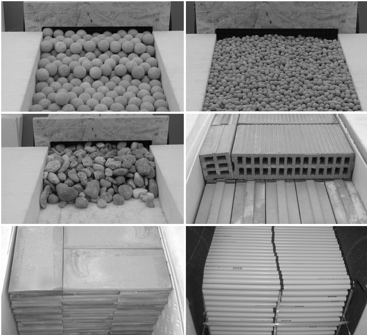
Figure $4 : Prototype filled with different storage materials. Top: ceramic spheres of two distinct sizes; Middle: gravel, perforated bricks; Bottom: ceramic slabs, pvc tubes filled with water.
