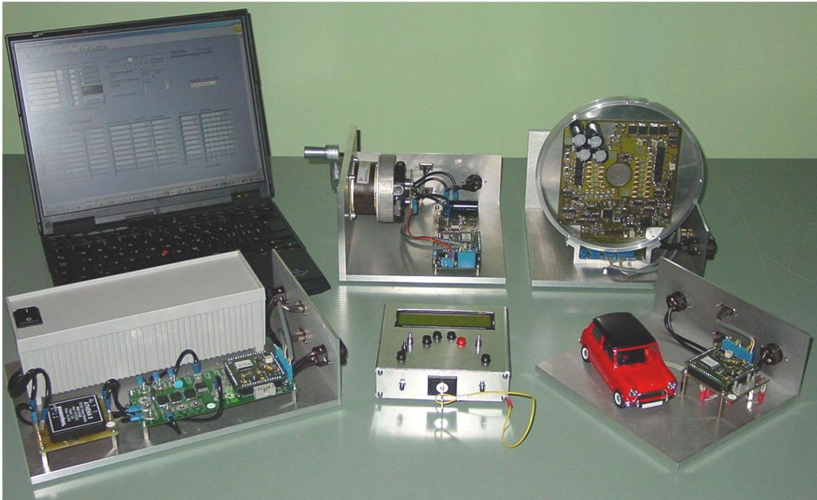
Figure 1 The demonstration-version of the control system shown consists of all kinds of modules needed to build a series-hybrid vehicle with one single motor.
