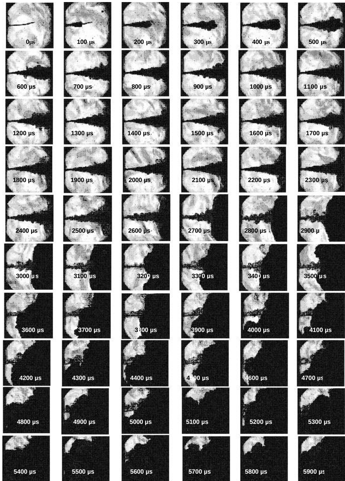
Figure 4: Injection sequence for T_{\text{cell}}=750\text{K} , p_{\text{cell}}=40\text{bar} , p_{\text{ini}}=500\text{bar} , t_{\text{ini}}=2.0\text{ms}
