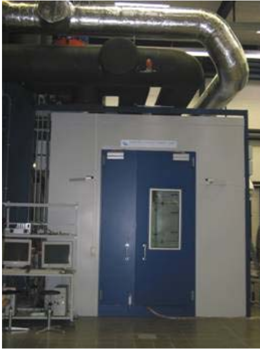
Fig. 7: Acoustic chamber for tests (left) and test equipment (right) of the HTA test rig
