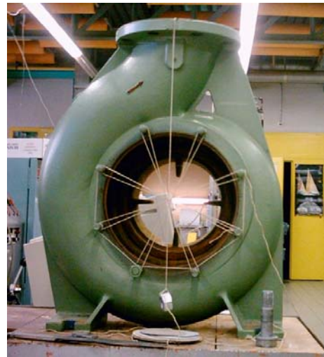
Figure 13: Volute geometry measurements
