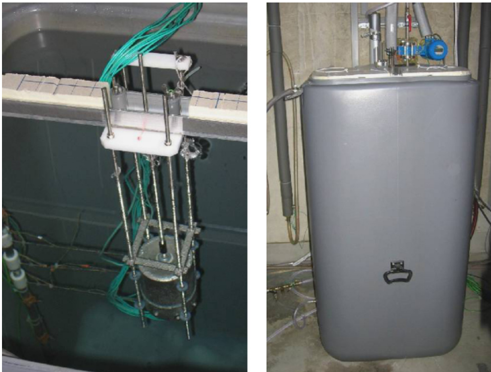
Fig. 12. PCM container plunged in a water tank.
