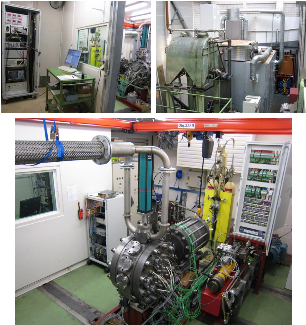
Figure 1: Final setup of the experimental spray combustion chamber test facility: control room (upper left), view from outside (upper right) and the experimental laboratory (lower image) itself.
