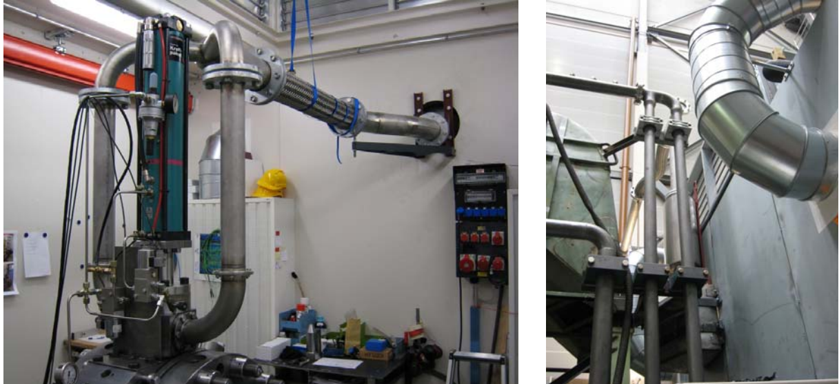
Figure 2: Exhaust system views inside and outside of the laboratory.
