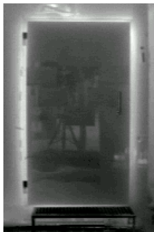
Figure 3.2c. Infrared picture of the test cell door.
