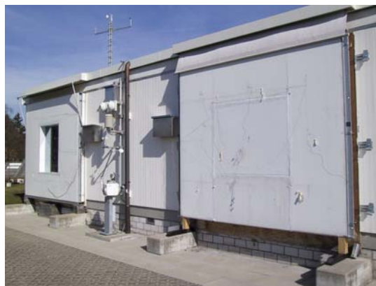
Figure 4.1b. Outdoor test facility with removable façade element.
