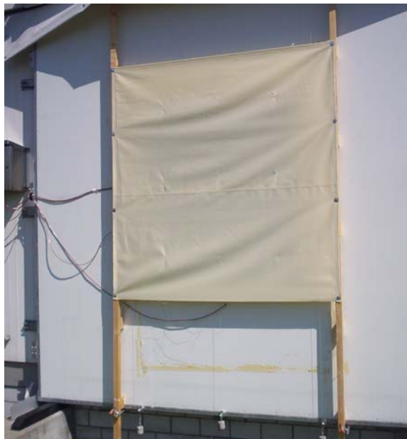
Figure 7.1. Photograph of the exterior shade mounted on the test cell.
