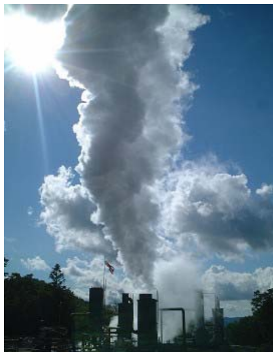
Figure 14.4 Production test for exploration well in Appi (North side of Honshu) geothermal field, research activities under Survey Program C conducted by NEDO, started from FY2000 to FY2003. Flowing rate : Steam 50t/h, water 0t/h (August 2003)
