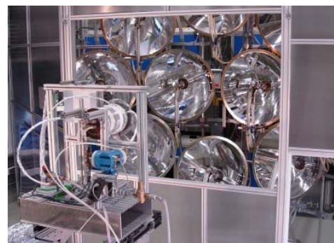
Figure 4: PSI's High-Flux Solar Simulator (HFSS) comprises an array of ten 15 kW e high-pressure Xenon arcs, each close-coupled with truncated ellipsoidal specular reflectors of common focus [20]. This facility is able to deliver a total radiative power of 50 kW with a peak radiative flux exceeding 10,000 suns. The total radiative power intercepted by a 6 cm diameter circular target – representing the reactor's aperture – is 20 kW, and the average radiative power flux over this aperture is more than 7,000 suns.
