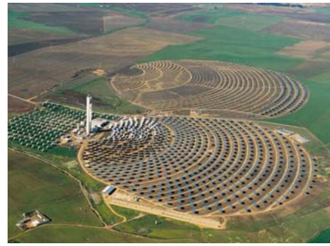
Figure 1: Left: schematic of the concentrating solar power (CSP) tower or “tower top” system. Right: aerial view of the 11 MW e thermoelectric plant PS10 in operation (foreground) and the 20 MW e plant PS20 under construction (background) near Seville, Spain [16],[17]. www.solucar.es
