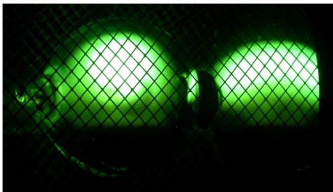
Figure 6 After evaporation of sulphur, modulation OFF (470 W)
