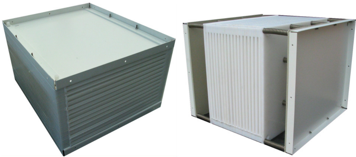
Figure 25 - Assembled membrane contactors: Left the absorber, right the desorber (Photos Empa).
