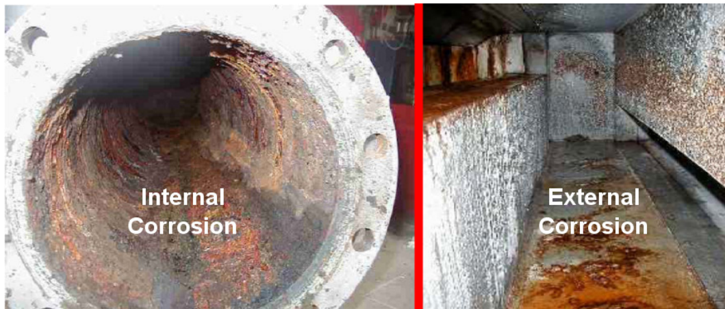
Figure 5 - Corrosion in open absorption systems: Left, in the condenser; Right, in the supply air channel. Adapted from [28].
