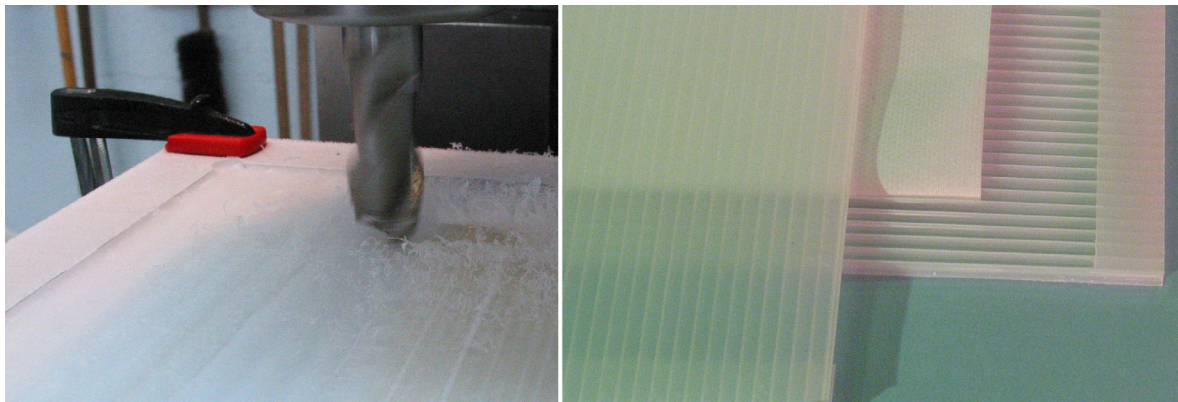
Figure 30 - Processing twin-wall structured plates: Left, milling the top wall; Right, plates after processing (Photos Empa).
