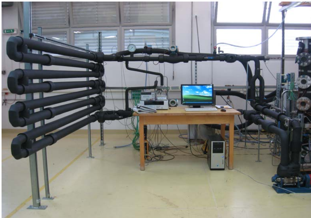
Fig.6: The pilot CO 2 hydrate slurry test rig
