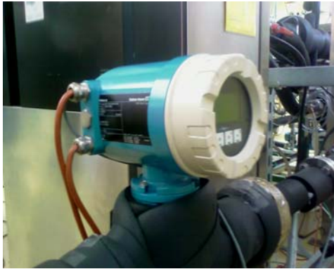
Fig.11: Endress+Hauser Mass flow meter to measure mass flow rate and density
