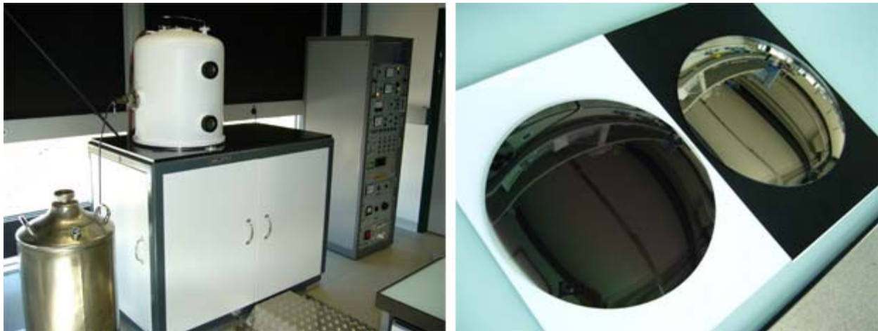
Fig. 4: Vacuum evaporation system (left). Black absorbing and mirrorlike film samples (right)
