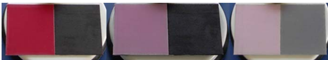
Fig. 7: Thermochromic paint samples at 25, 40, and 90°C
