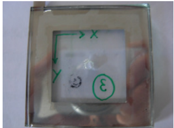
Fig. 5 b) 250 \mu m Al-sheet specimen
