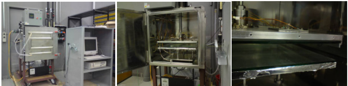
Fig. 36 Images showing the entire prototyping system including controls (left), the interior of the HV chamber (center) and the heated Al electrodes with mounted glass panes (right).
