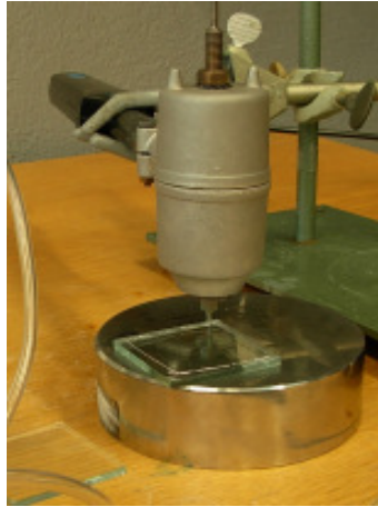
Fig. 26 Photographic image of the liquid solder dispenser operating in air
