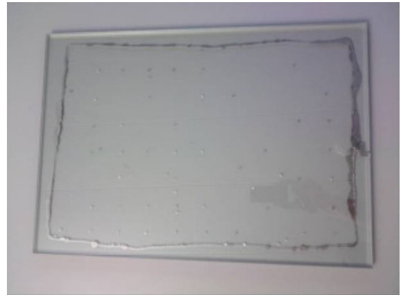
Fig. 38 First 50 cm by 30 cm sealing prototype manufactured in the large high vacuum chamber.
