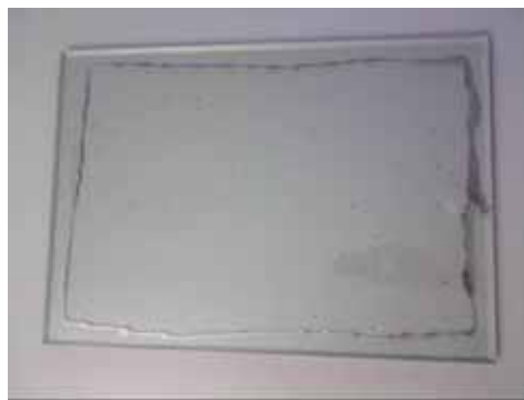
Fig. 6: First 50 cm by 30 cm sealing prototype manufactured in the large high vacuum chamber.
