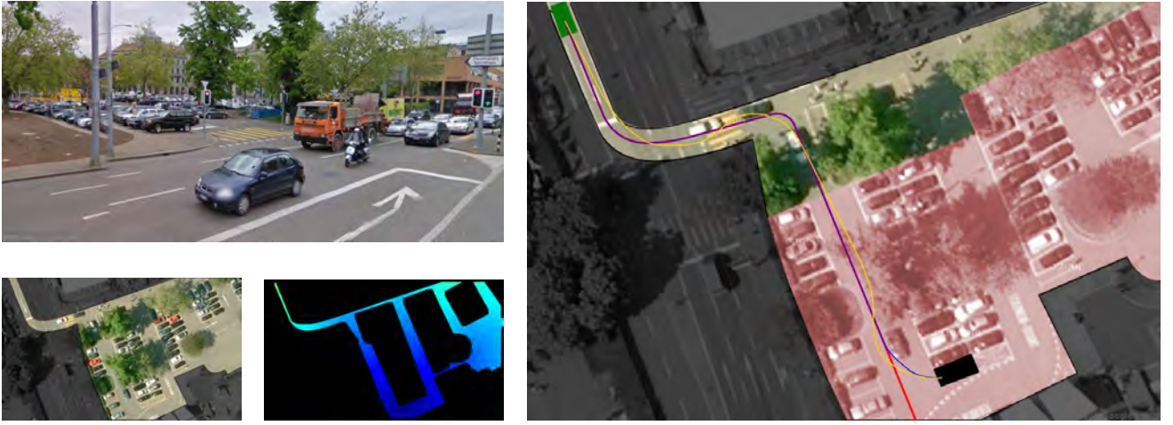
Fig. 4. Top Left: Google Street View scene close to Bellevue, Zurich. Bottom Left: corresponding Google Maps image. Impassable areas are shaded gray. Bottom Center: 2D heuristic map. Color indicates cost to goal. Right: plan from start- (green) to goal-configuration (black). The lattice shape (at d = 0 ) is displayed in red. Note that the curvature is set to zero in the parking lot area due of lack of structure in close vicinity. Instead, the direction is aligned with the dominant orientation of the lot area. The solution on the deformable lattice is represented in blue, the one on the fixed lattice in yellow.
