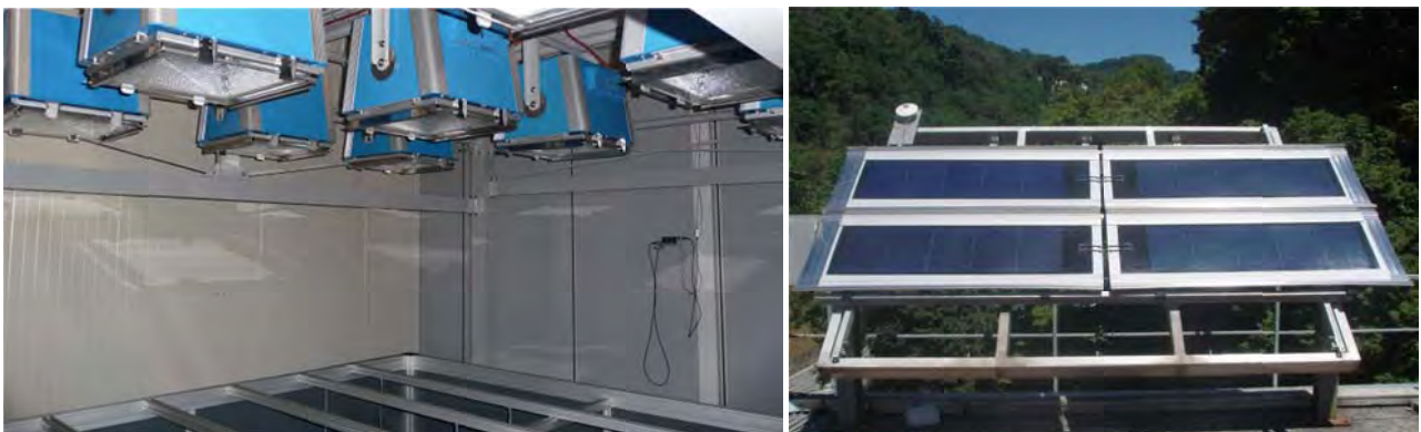
Figure 5. Light soaking facilities for PV modules. Left: Steady-state sun simulator. Right: outdoor stand for sunlight exposure.
