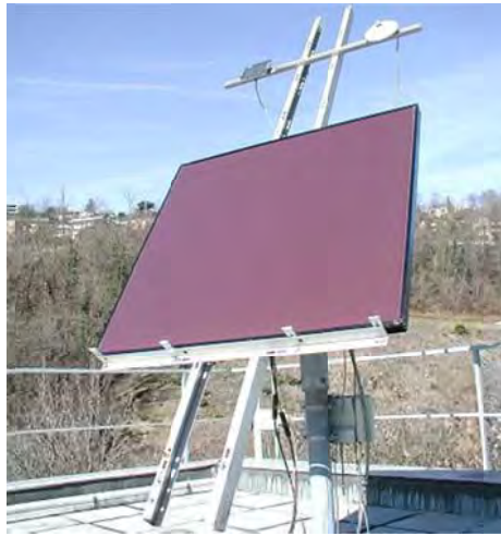
Figure 8. Suntracker system for outdoor IV-curve measurement. Irradiation data are collected by means of a pyranometer and a c-Si reference cell. A temperature sensor (PT100), attached to the back of the module, is used to monitor module temperature
