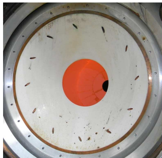
Figure 3: Frustum-shaped water-cooled front cone coated with ceramic ZrO 2 /Al 2 O 3 layer. To protect the window from precipitations, inert gas (Ar) is injected through 24 radial nozzles at the window and 12 tangential nozzles on the cone.
