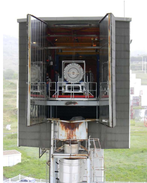
Figure 9: Solar pilot plant mounted on mobile carriage (left) in solar tower experimental platform of MWSF, Odeillo, France (right). Remark that the radiation shield has not been mounted yet.
