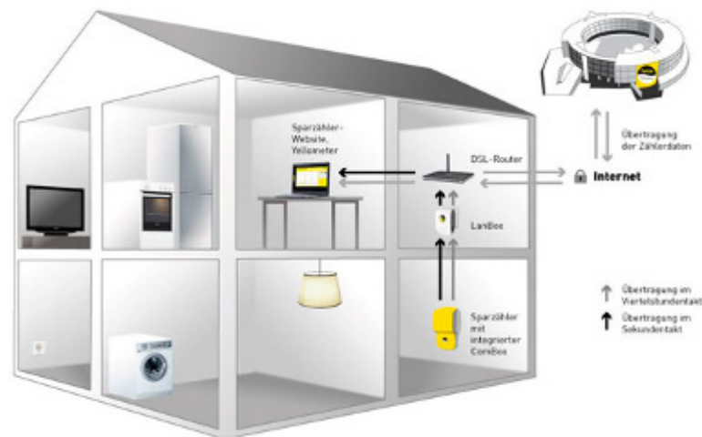
Figur 60: YelloStrom System (Quelle: YelloStrom)
