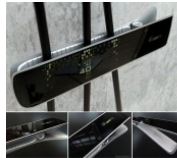
WattBlock disconnects devices when you step on them.
