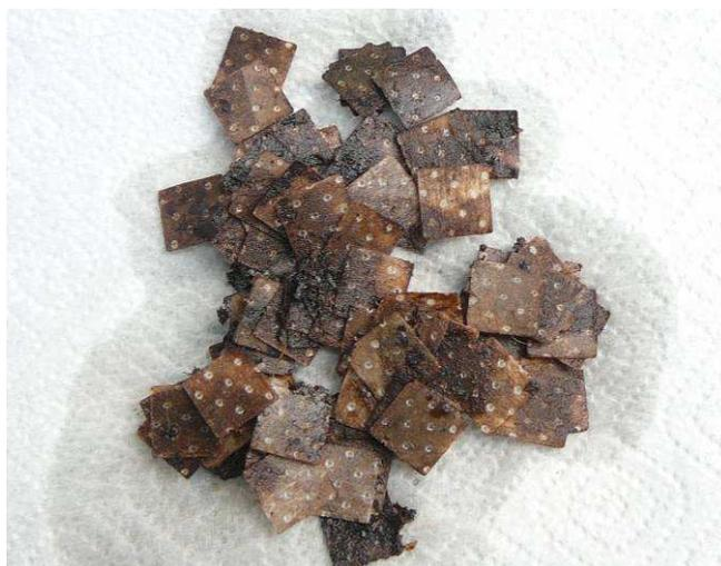
Figure 3-2 : Support mobile FLUOPUR couvert de biofilm
